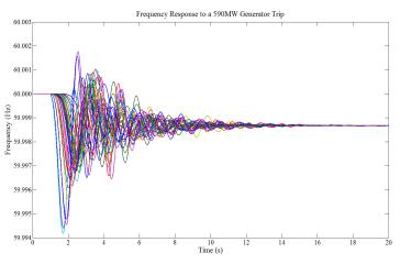
Fig. 1 2030 high wind scenario: 590 MW generator trip (detailed 70,000 bus model)
