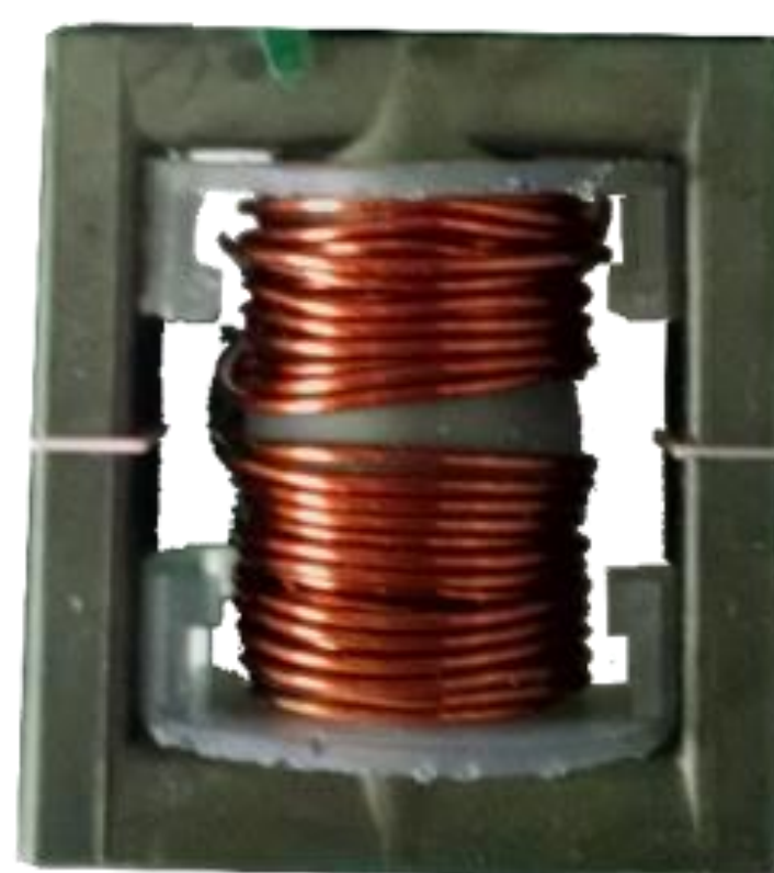
Figure 5: Designed Inductor with Proposed Bobbin
