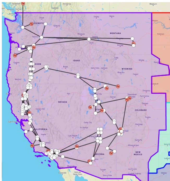
Fig. 9. WECC 179-bus system visualized in CURENT LTB.
