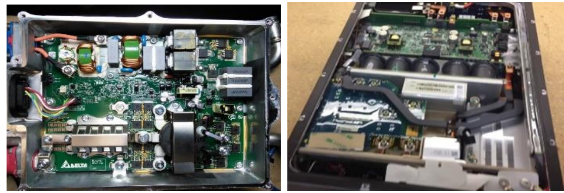
Fig. 1. Standalone Units: APM of Tesla Model 3, & OBC of Model S.
