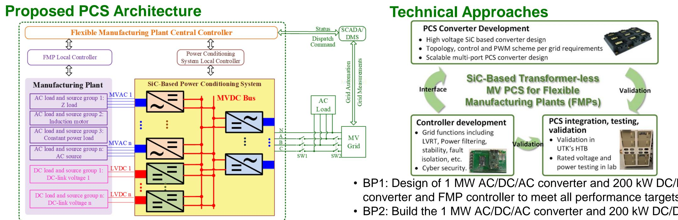
A scalable multi-port MW-scale SiC based PCS and control for manufacturing plants to enable increased FMP dispatchability, resiliency, and grid support functions.
