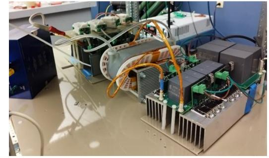
10 KV SiC MOSFET based dual active bridge (DAB) converter unit
