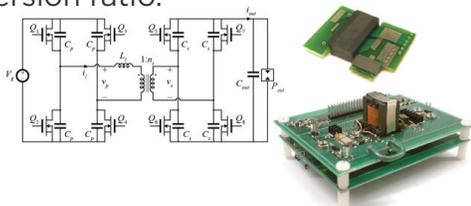
Wide bandgap devices are being assessed analytically and experimentally to determine the degree of benefit which can be obtained through the use of new semiconductor materials.
