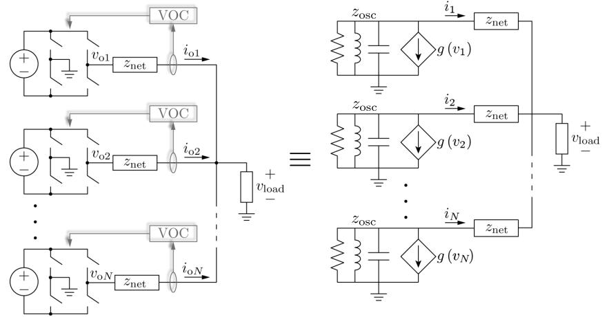
Condition for global asymptotic synchronization  $\sup_{\omega \in \mathbb{R}} \left\| \frac{z_{\text{net}}(j\omega) z_{\text{osc}}(j\omega)}{z_{\text{net}}(j\omega) + z_{\text{osc}}(j\omega)} \right\|_{2} \sigma < 1$
