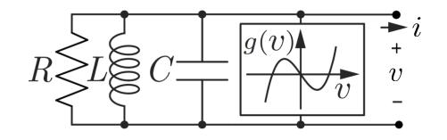
$\frac{d^2v}{dt^2} + \left(\frac{1}{RC} - \frac{g'(v)}{C}\right)\frac{dv}{dt} + \frac{v}{LC} = -\frac{1}{C}\frac{di}{dt}$
