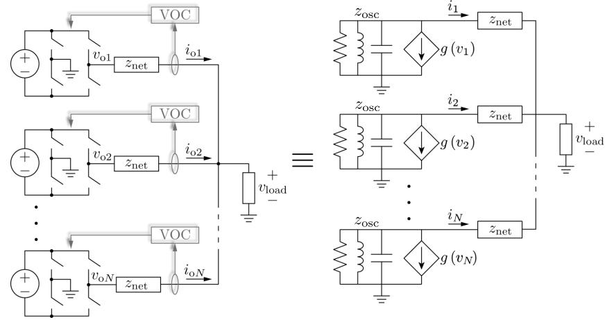
$\begin{array}{ll} \text{Condition for global asymptotic synchronization} & \text{Modular} \\ \sup_{\omega \in \mathbb{R}} \left\| \frac{z_{\text{net}}(j\omega) z_{\text{osc}}\left(j\omega\right)}{z_{\text{net}}(j\omega) + z_{\text{osc}}\left(j\omega\right)} \right\|_{2} \sigma < 1 & \text{Robust} \\ \end{array}$
