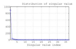
Fig. 4 - Singular values of a 600 × 37 PMU data matrix
