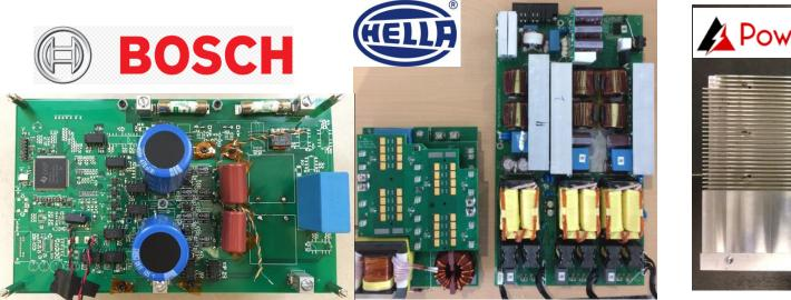
DC-grid non-isolated charger, 2013 6.6kW charger (GaN vs Si), 2015
