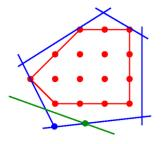
• If the solution to the linear relaxation is outside of the convex hull, add a linear constraint that will remove it from the relaxation.
