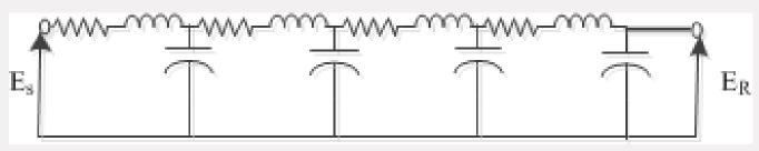
Lines are also represented with lumped parameters where the line capacitances are split between two ends.
