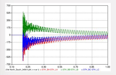
b. With both shunt reactors connected and utilization of 4250hm pre-insertion resistors inserted for 13ms
