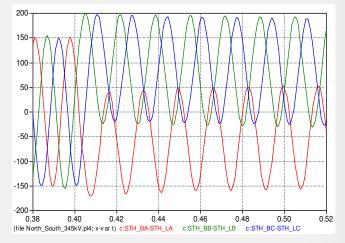
South line end current following energization of South line-end shunt reactor on a closed through transmission line with North lineend reactor connected. Approx. 46 MW are flowing on the line
