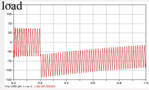
ATP Simulation -Line breaker Current (A-Ph) with No load
