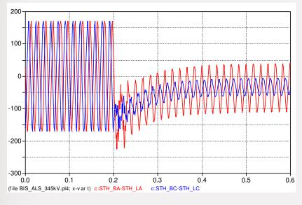
Line breaker currents on unfaulted phases
