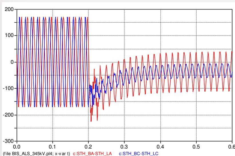
Line breaker currents on unfaulted phases
