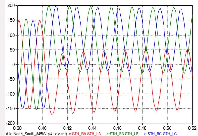
South line end current following energization of South line-end shunt reactor on a closed through transmission line with North line-end reactor connected. Approx. 46 MW are flowing on the line
