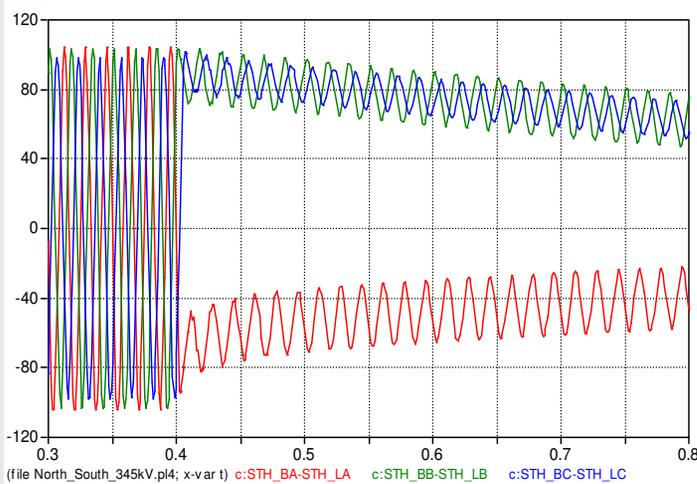
South Substation line breaker current following uncontrolled closing of South line-end reactor with limited power flow on the line
