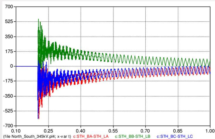
b. With both shunt reactors connected and utilization of 425ohm pre-insertion resistors inserted for 13ms
