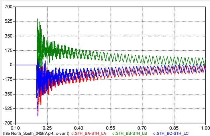
b. With only north end reactor connected
