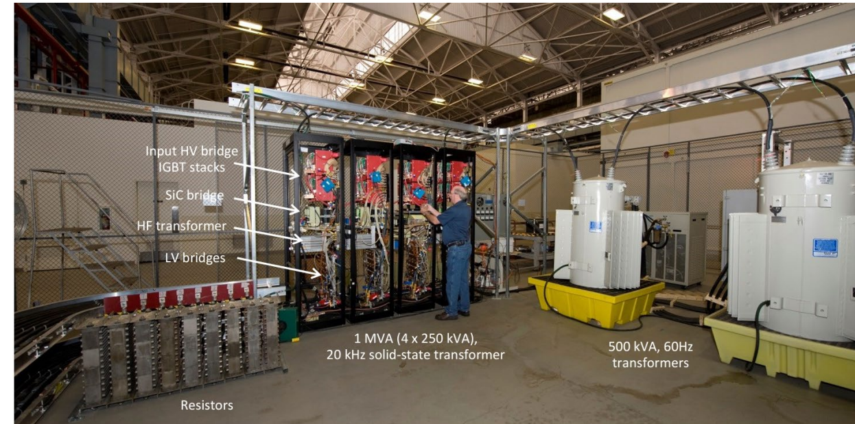
Fig. 4. Back-to-back test setup with prototype SST cabinets and 60 Hz transformers.
