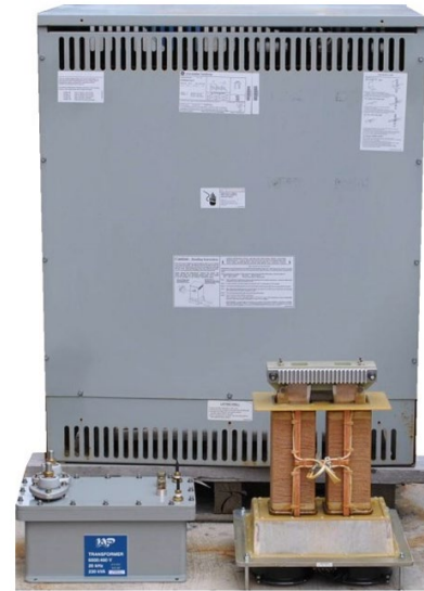
Fig. 2. ~250 kVA transformers – 60 Hz dry-type (back), 20 kHz oil-filled er-cooled (front left) and 20 kHz dry-type forced-air cooled (front right).
