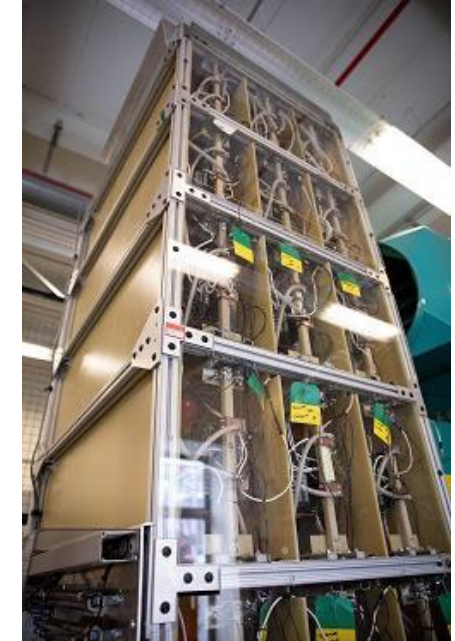
1MW, 6kVac – 690Vac 200kHz SST (2021)
