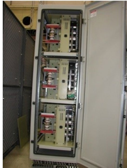
1MW, 4.16kVac – 1kVdc 40kHz SST (2011)
