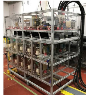
1MW, 6kVdc – 1kVdc 200kHz SST (2020)
