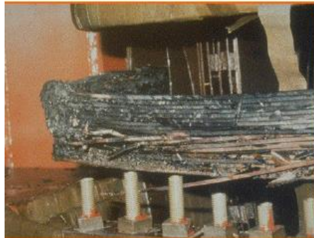
Evidences of transformer overheating due to GIC flow in 1989 at Salem Nuclear plant, NJ (left) and in 2003 at the Eskom station in South Africa (right). Source: [9]
