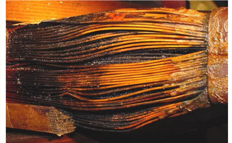
Evidences of transformer overheating due to GIC flow in 1989 at Salem Nuclear plant, NJ (left) and in 2003 at the Eskom station in South Africa (right). Source: [9]
