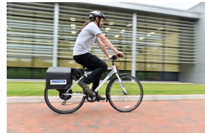
FARADION: Na-ion battery powered vehicle
