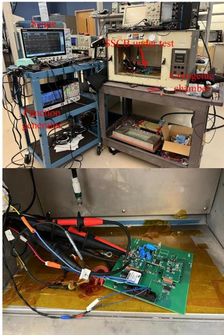
Fig. 10. Cryogenic test set up for the proposed SSCB.
