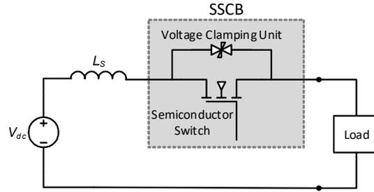
Fig. 2. Typical SSCB in a DC system
