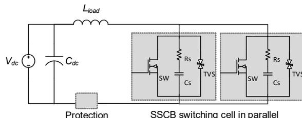
Fig. 8. Circuit diagram for testing paralleled GaN HEMTs.
