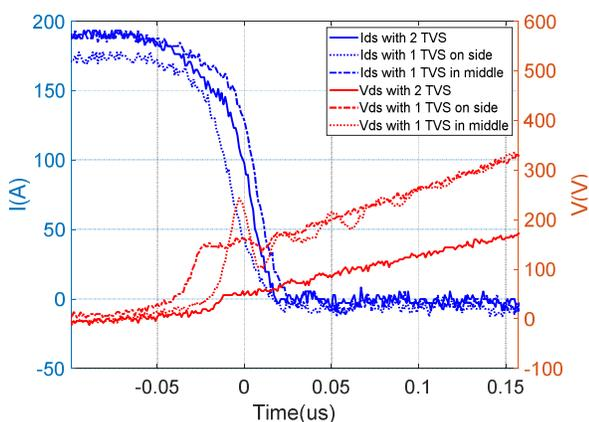
Fig. 7. Turn-off waveforms with different TVS configuration.
