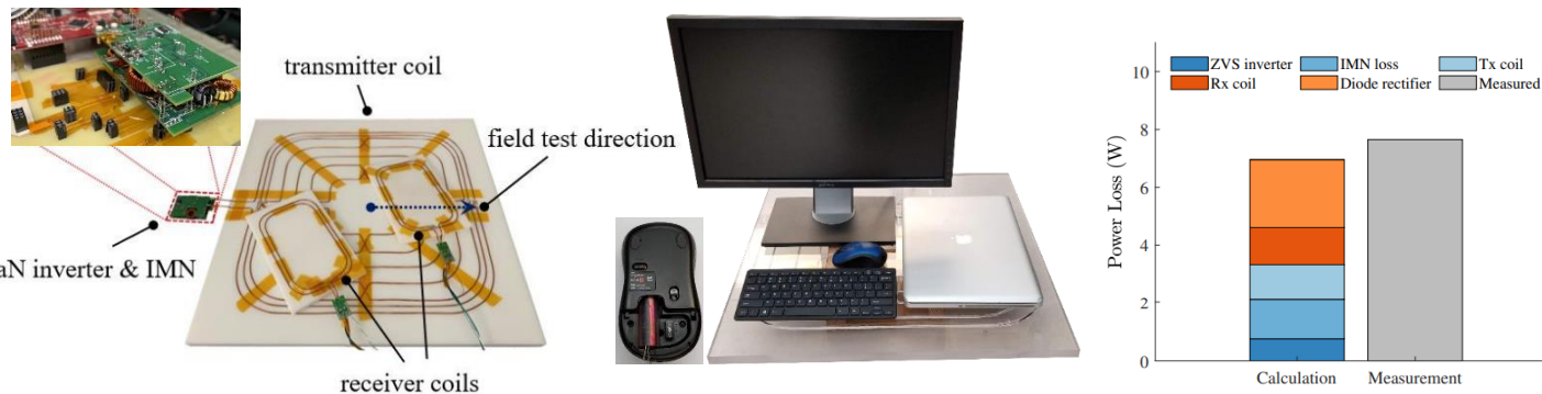
Multi-receiver 100 W workstation with 92% end-to-end efficiency
