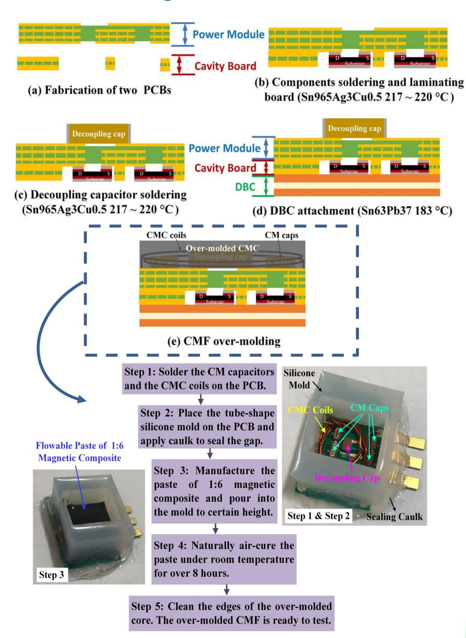
The over-molded CM choke (CMC) cures under room temperature, with no pressure, thus highly package-compatible.
