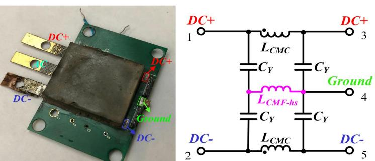
The impedance of the filter is **measured** by network analyzer and curve-fitted to obtain each parameter.
