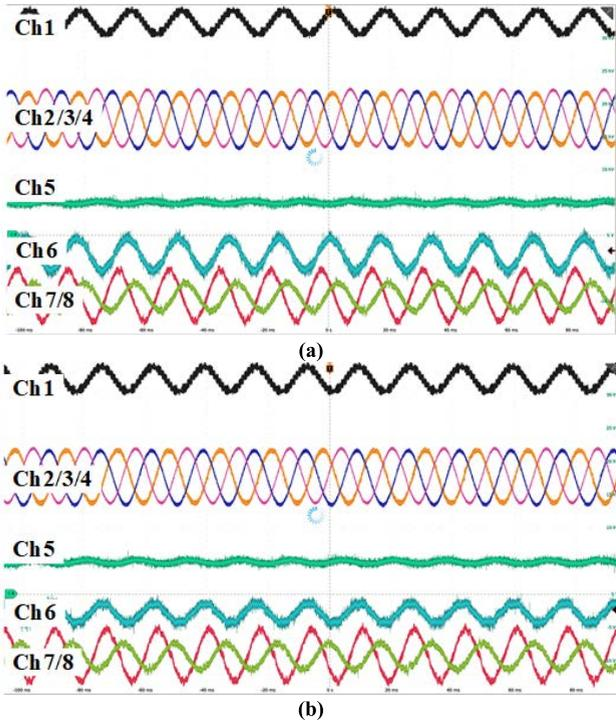
**FIGURE 21.** Microgrid side unbalanced load support operation test results: Ch1, grid voltage (10 kV/div); Ch2/3/4, microgrid voltage (5 kV/div); Ch5, dc link positive voltage (5 kV/div); Ch6, grid current (2 A/div); Ch7/8, microgrid current (5 A/div). (a) without zero-sequence and negative-sequence control; (b) with zero-sequence and negative-sequence control.
