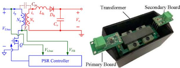
FIGURE 12. The isolated power supply schematic and prototype.
