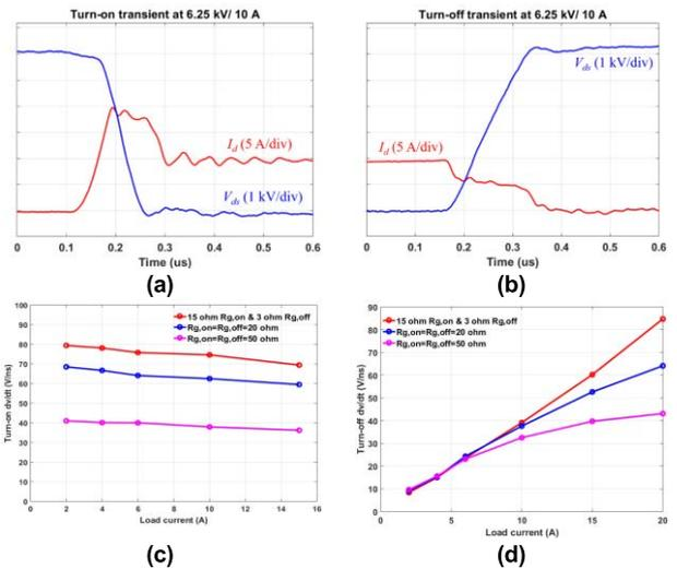
FIGURE 8. Switching characteristics of 10 kV SiC MOSFET at 6.25 kV and 125 °C. (a) turn-on transient, (b) turn-off transient, (c) turn-on  $dv/dt$  and (d) turn-off  $dv/dt$ .
