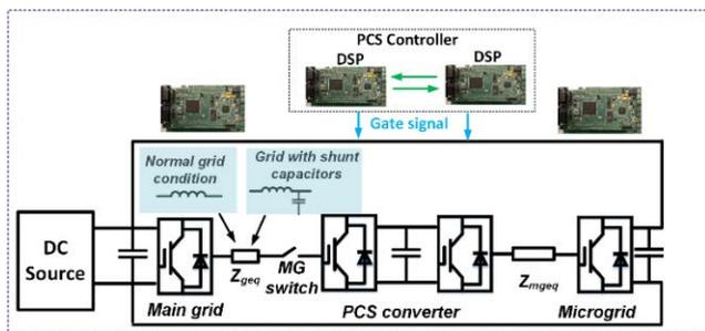
**FIGURE 26.** ASMG HTB testing setup.
