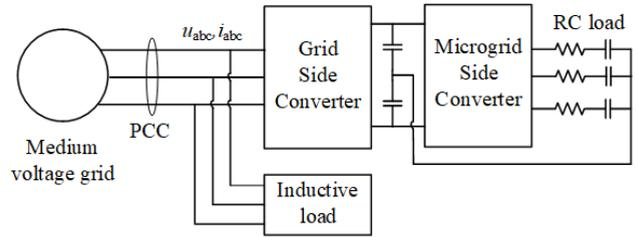
**FIGURE 22.** Reactive power compensation test circuit.
