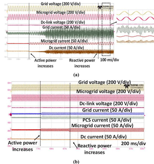
FIGURE 29. PCS grid stability enhancement testing: (a) 4 kHz control frequency; (b) 10 kHz control frequency.
