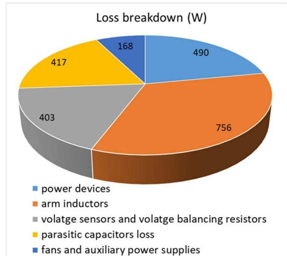
FIGURE 20. Loss breakdown of the PCS converter at rated voltage and full load.
