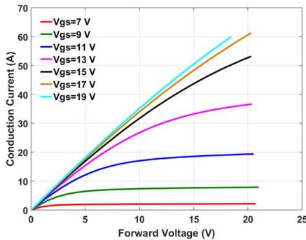
FIGURE 6. Forward I-V characteristic of the 10 kV SiC MOSFET at 25 °C.
