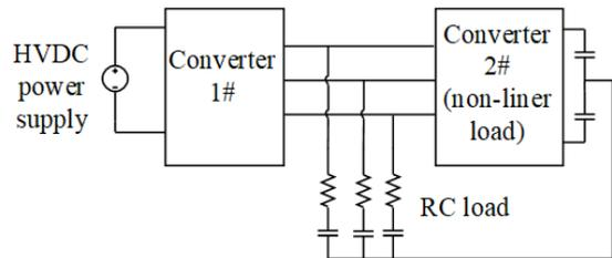
**FIGURE 24.** Active power filter test circuit.
