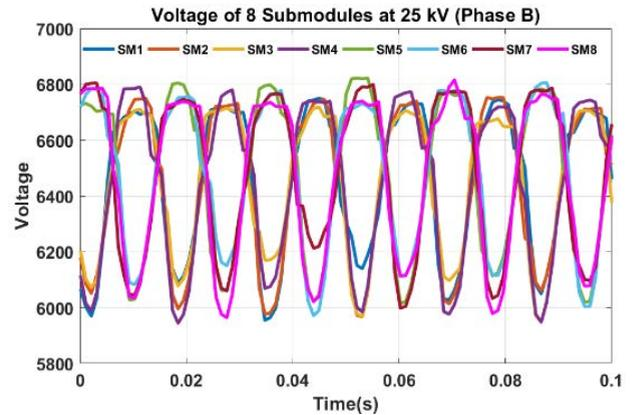
FIGURE 17. Submodule voltage balance control test results.
