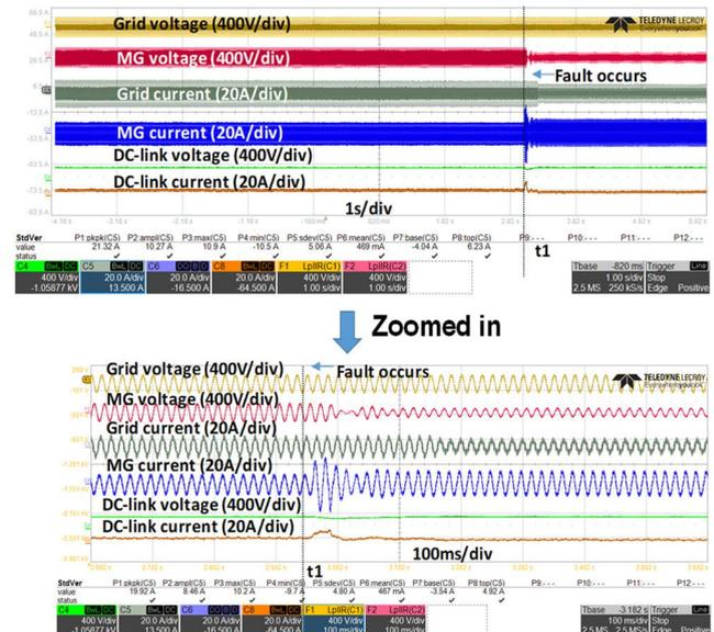
**FIGURE 27.** Testing results of PCS fault ride through in the grid-connected mode.
