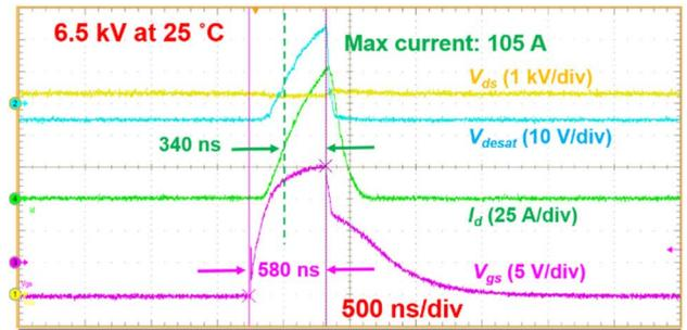
FIGURE 11. HSF short circuit test of the lower MOSFET in MMC submodule at 6.5 kV dc bus voltage.
