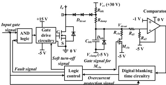
FIGURE 10. Desat protection circuit of the 10 kV SiC MOSFET.
