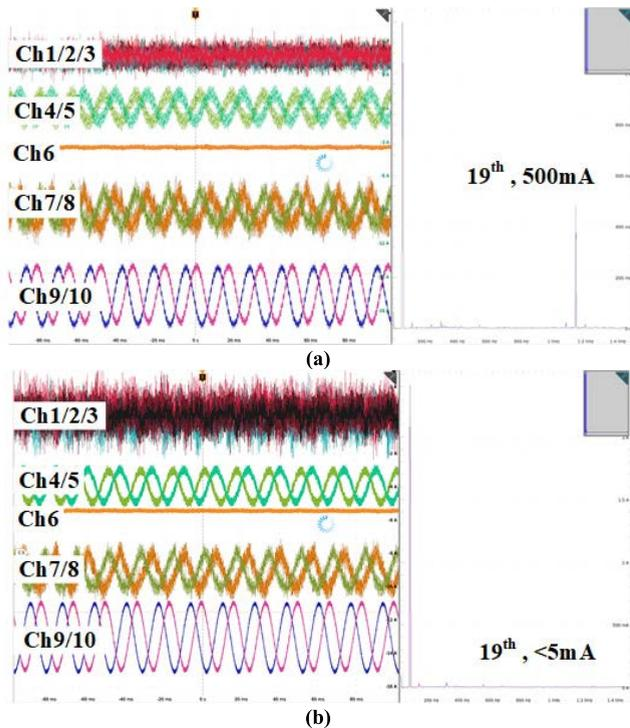
**FIGURE 25.** Active power filter experimental results: Ch1/2/3, rectifier mode converter output current (5 A/div); Ch4/5, RC load current (5 A/div); Ch6, rectifier mode converter dc link voltage (10 kV/div); Ch7/8, inverter mode converter output current (5 A/div); Ch9/10, grid voltage (10 kV/div). (a) without harmonic filter; (b) with harmonic filter.
