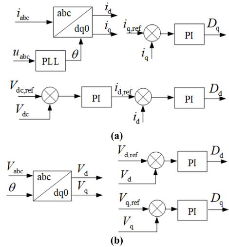
FIGURE 16. Control diagram of the back-to-back PCS converter system, (a) grid side converter and (b) microgrid side converter.
