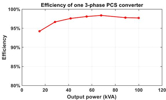
FIGURE 19. Efficiency curve of the PCS converter.
