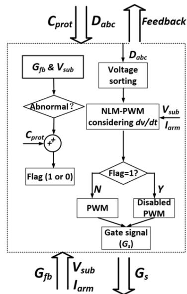
FIGURE 4. PCS converter single phase controller function block diagram.
