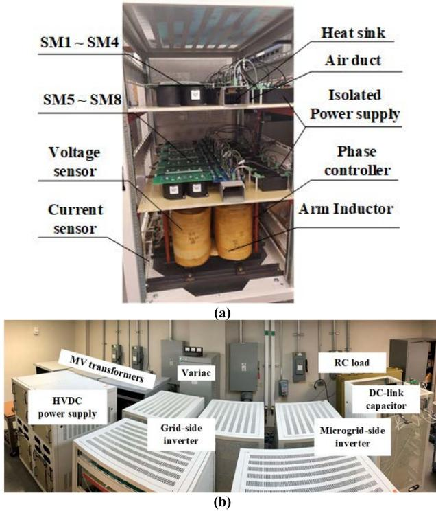
FIGURE 14. (a) One phase-leg hardware, (b) test setup of the back-to-back PCS.
