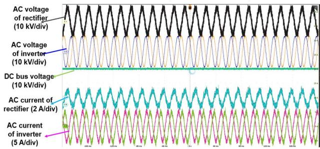
FIGURE 18. Test results of the back-to-back PCS at rated voltage and power.
