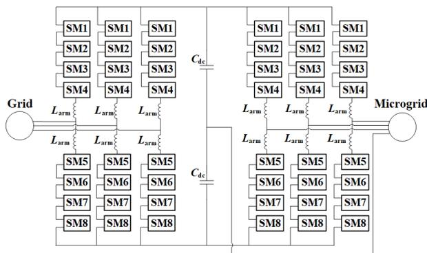
FIGURE 2. Overall structure of the MMC-based PCS.
