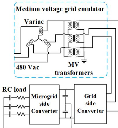
FIGURE 15. Back-to-back structured test circuit of the PCS converters.
