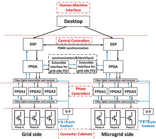
FIGURE 3. ASMG PCS control architecture.
