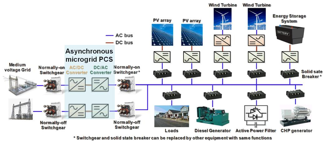
FIGURE 1. Configuration of a MV ASMG.
