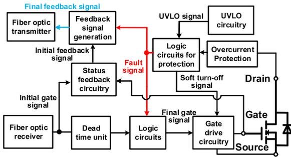
FIGURE 9. Function diagram of the designed 10 kV SiC MOSFET gate driver.
