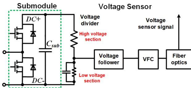
FIGURE 13. Block diagram of the designed submodule voltage sensor.
