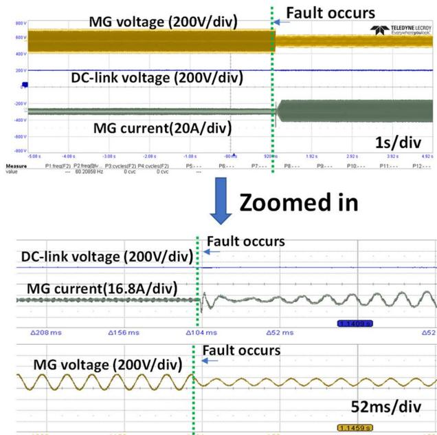
FIGURE 28. Testing results of PCS fault ride through in islanded mode.
