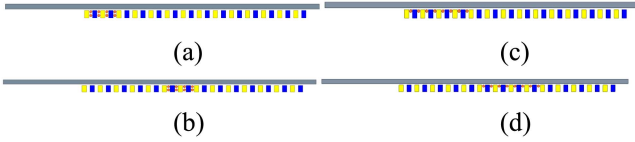
Fig. 6. Examples of the LV coils with different arrangements and positions. (a) Vertical, LV position = 0. (b) Vertical, LV position = 10. (c) Horizontal, LV position = 0. (d) Horizontal, LV position = 10.
