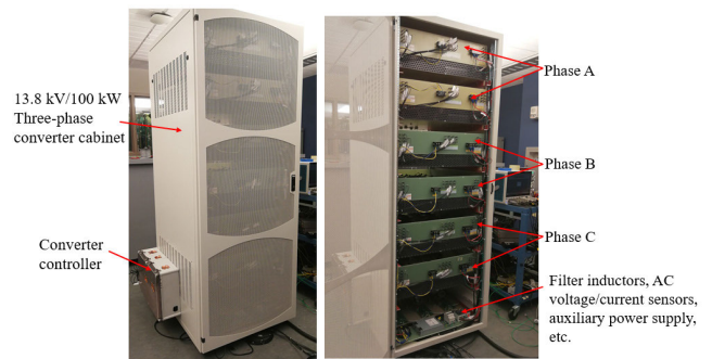
FIGURE 18. The three-phase converter prototype.
