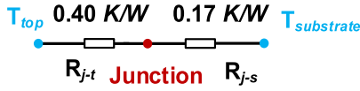
Fig. 4. Thermal model of lateral GaN HEMT (GS-065-060). R_{j-s} is the thermal resistance from junction to substrate. R_{j-t} is the thermal resistance from junction to top.
