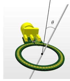
Fig. 6. Tilted primary-side conductor in Rogowski coil.
