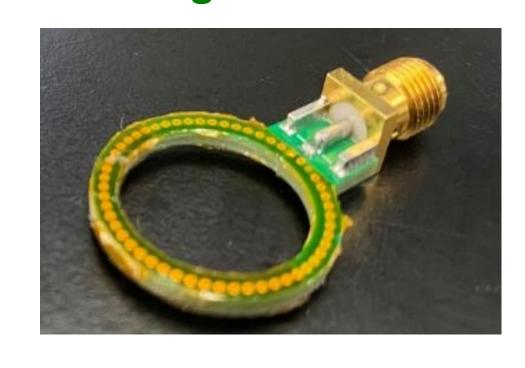
$$\frac{V}{I} = \frac{M}{L_S} \times \frac{1}{R_l^{-1} - j\sqrt{C_S/L_S}\cot(\omega\sqrt{L_S}C_S)}$$
