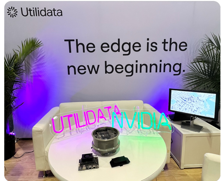
At DISTRIBUTECH International 2024, from left to right: an NVIDIA Jetson developer kit, Utilidata's meter collar, and 3D print model of Utilidata's custom module
